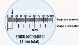
3. With a STAGE MICROMETER, you can determine how much 10 EGU are equivalent to (CALIBRATION). Here: 0.008mm (8um).
